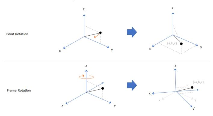
Orientation is defined as the frame rotation that takes the parent frame to the child frame. The choice of parent frame depends on the problem space. For example, manipulating sensor frames is necessary to align various axes of independent sensors. Tracking the body frame is often used for stabilization tasks. The ground reference frame is useful for tracking multiple independent platforms and locating platforms in an absolute sense.
