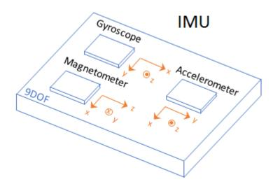
With this toolbox, measurements returned from an IMU model use the following unit and coordinate conventions.
