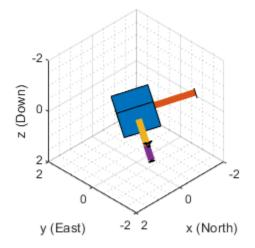
Note that the **ecompass** algorithm correctly finds the location of north. However, because the function is memoryless, the estimated motion is not smooth. The algorithm could be used as an initialization step in an orientation filter or some of the techniques presented in the "Lowpass Filter Orientation Using Quaternion SLERP" could be used to smooth the motion.
