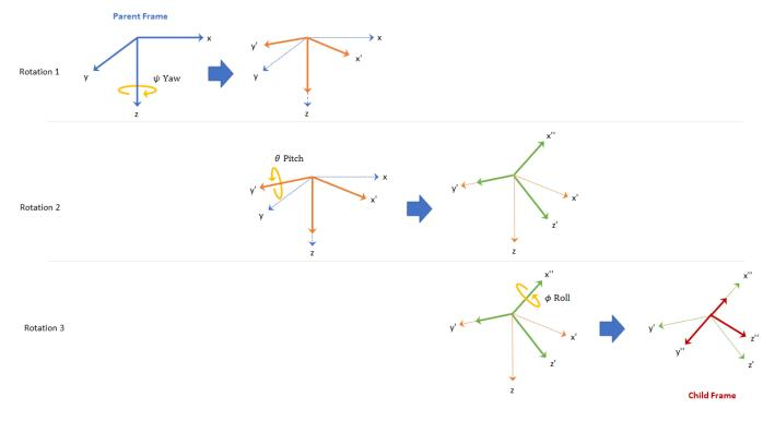
This sequence of rotations follows the convention outlined in [1]. The rotation matrix required to convert a vector in the parent frame to a vector in the child frame for a given yaw, pitch, and roll is computed as:
