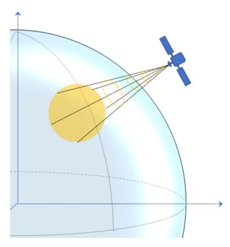
GPS consists of a constellation of satellites that continuously orbit the earth. The satellites maintain a configuration such that a platform is always within view of at least four satellites. By measuring the flight time of signals from the satellites to the platform, the position of the platform can be
